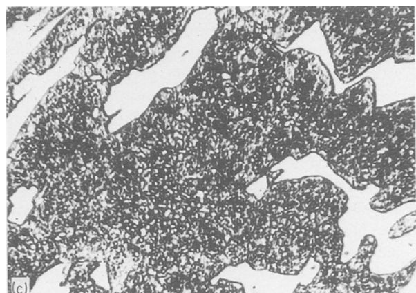
Figure 2 The structure of (a) the solidified melt zone; and of the hardened zone in (b) cast iron and (c) heat-treated iron × 3490.
